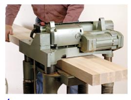
4 After truing one face of each piece with a hand plane, use a thickness planer to mill the opposite sides.
