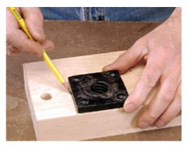
10 Before mounting the end-vise cap on the benchtop, install the threaded end-vise collars.
