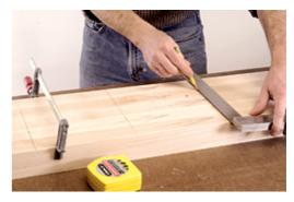
1 Clamp a group of benchtop strips together and lay out the locations for the joining-plate slots. Arrange the strips so that the grain runs in the same direction to facilitate planing the top after the pieces have been glued together.
