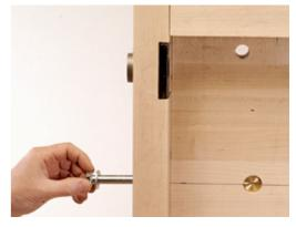
11 Join the end-vise cap to the top with bench bolts. Don't use glue. The top must be free to move.
