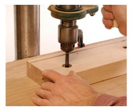
8 After routing a spline groove in each apron, bore stopped holes for the cylindrical bench-bolt nuts.
