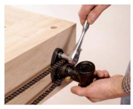
12 After adjusting the chain length, thread end-vise screws in place and attach outer vise collars.
