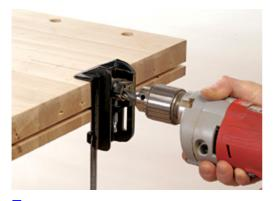
7 Bore holes in the ends of the top and aprons for securing the caps. Use a doweling jig to guide the bit.
