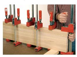
**3** Glue up three sections of five strips. Then, check to see if the sections are flat and straight.
