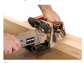
2 Use a plate joiner to cut slots at plate locations. Plates ensure good alignment between strips.
