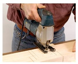
9 Lay out the cuts and mortises necessary for mounting the side vise. Use a sabre saw to cut the stock.
