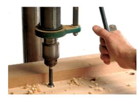
5 Lay out the bench-dog hole locations, and use a drill press and Forstner bit to bore the holes.
